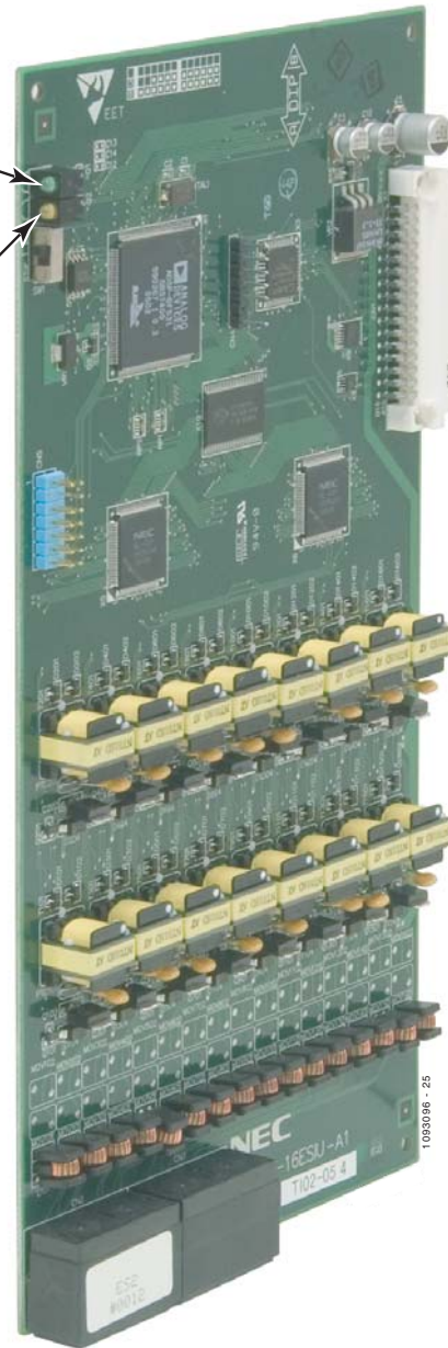
Figure 35: Digital Station (ESIU), Analog Station (SLIU), and Analog Line (COIU) Card LEDs
