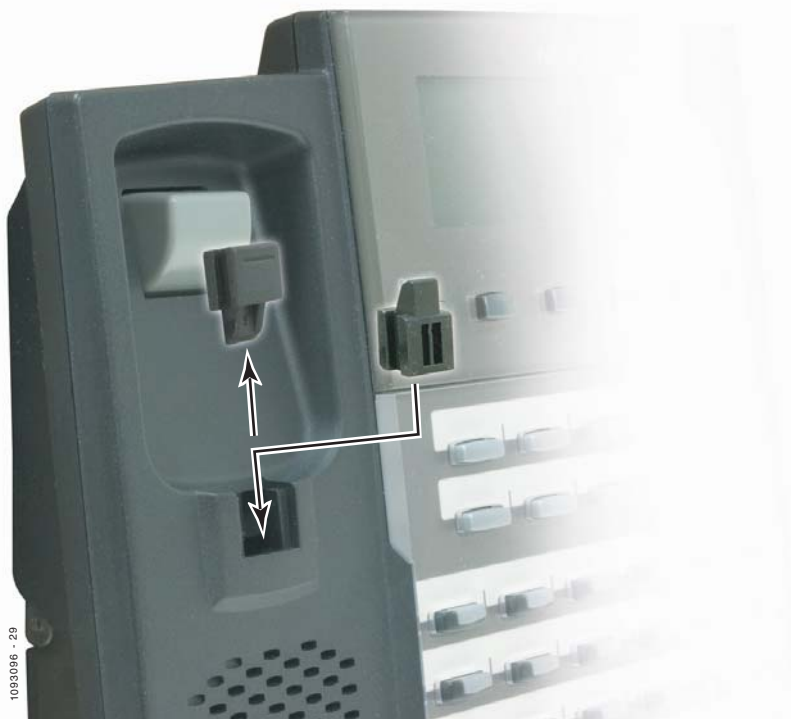
Figure 49: Reversing the Handset Hanger
