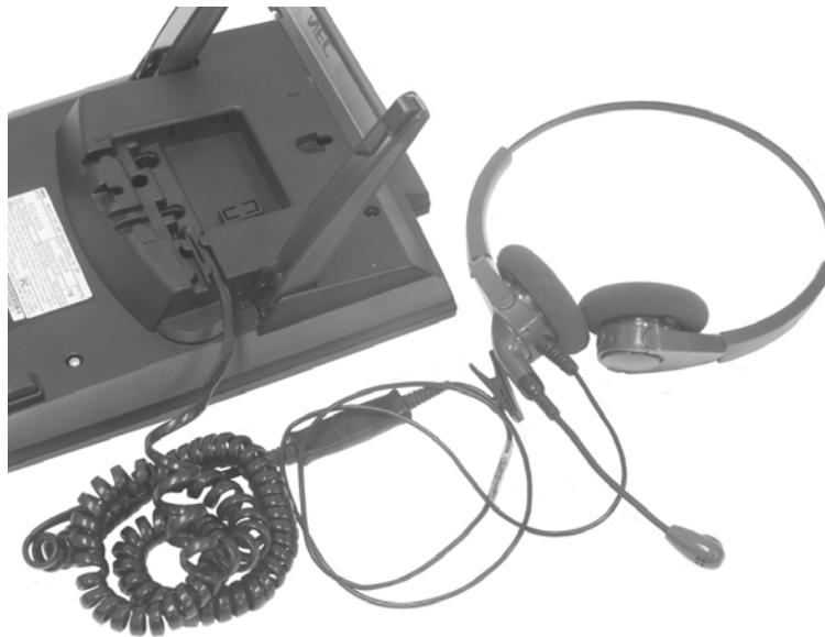
Figure 26: Installing the Optional Headset
