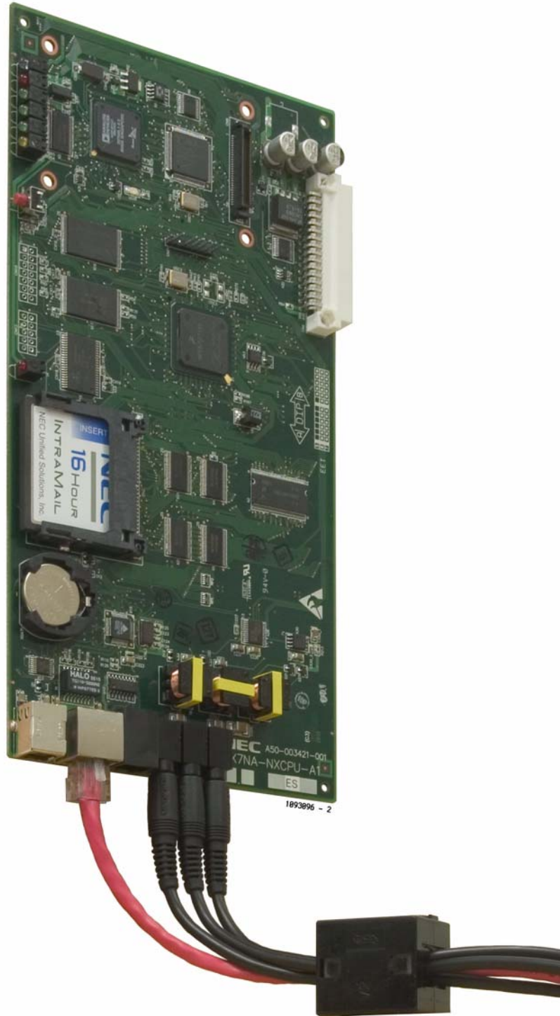
Figure 10: Installing the RFI Suppressor Assembly
