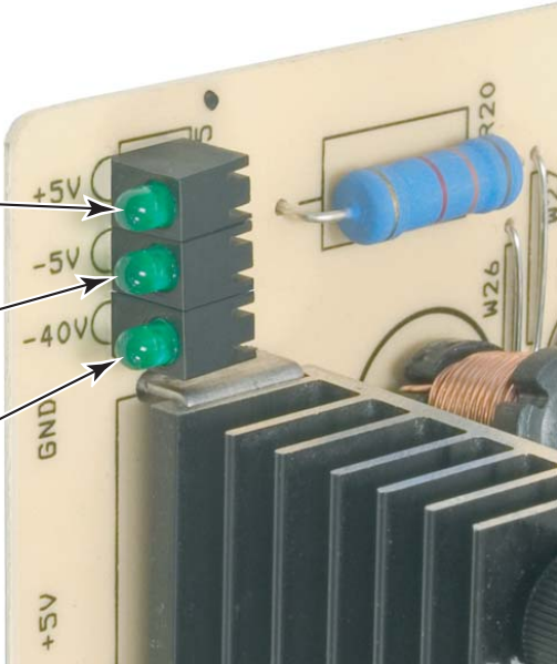
Figure 33: Power Supply LEDs
