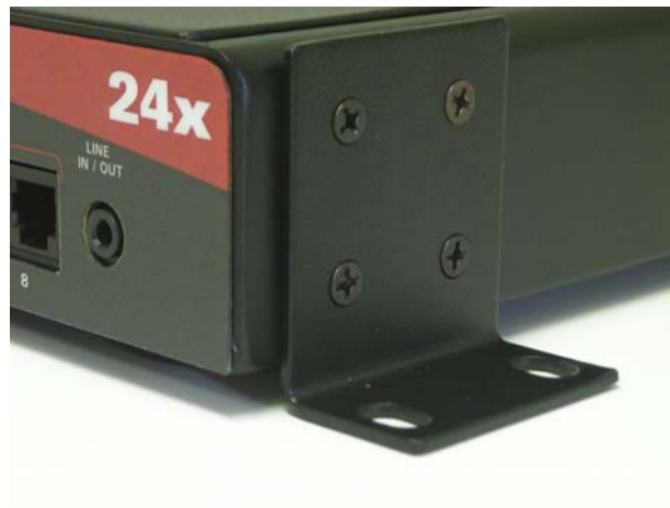
Figure 4: Wall Mount Bracket Installation
